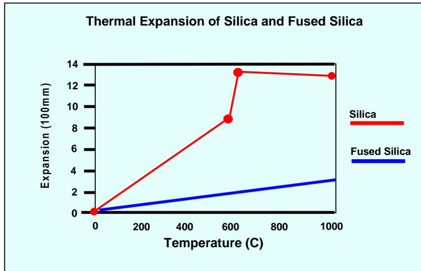
Materials with high density such as zircon and chromite sands can also improve the veining and surface finish of castings. Such high-density materials are also able to absorb a great amount of heat. Their expansion is quite low and little stress is developed. Unfortunately, these materials are rather expensive in comparison to silica sand. They are often 20 to 30 times the cost of silica sand and are used conservatively.
