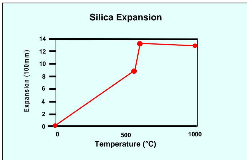
The previous chart shows initial heating of the sand causes a steady increase in the sand size up to approximately 1067°F (575°C). From this temperature to 1112°F (599°C), there is a sudden expansion of the sand. It is usually this sudden expansion that is the major cause of stress in sand mold components. Because the stress builds suddenly and is difficult to relieve quickly, it can lead to mold or core cracking, resulting in veining as shown earlier.
