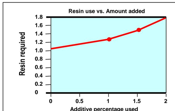
Although individual resin usage levels vary, this general trend is typical. It should be noted that increased resin usage promotes veining and several other defects, and merely accomplishes an increase in the handling strength. The use of burnout material can be an economical method of controlling veining. However, it can do little for reduction in or need for core washing.
